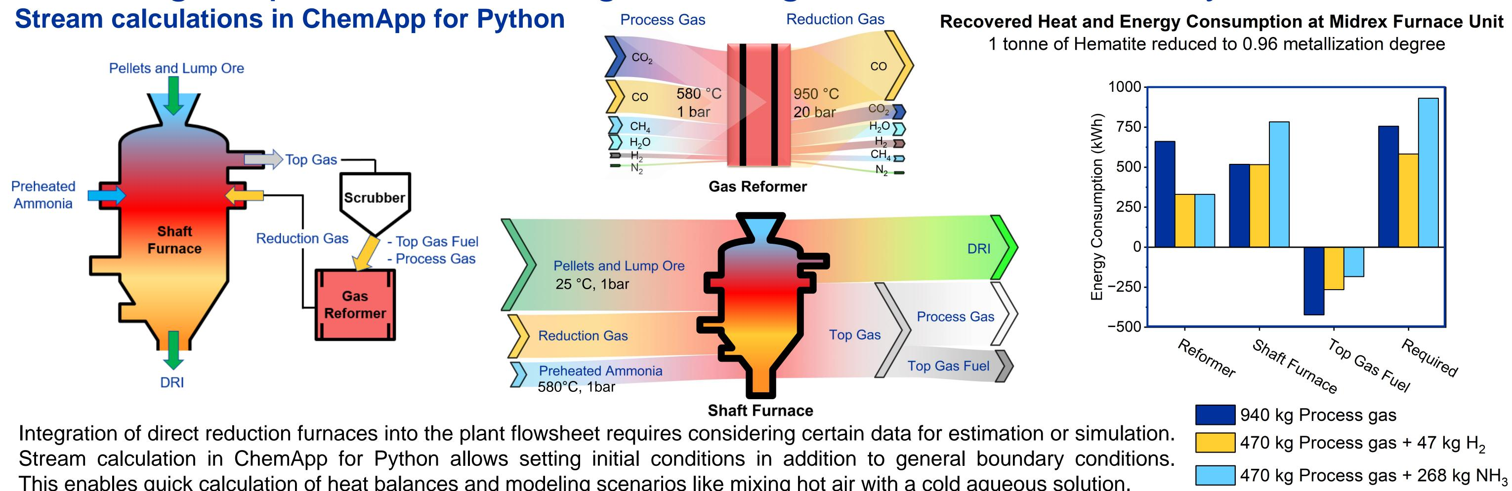
This enables quick calculation of heat balances and modeling scenarios like mixing hot air with a cold aqueous solution.
