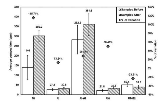
Average content of Si, S, soluble-Al, Ca e O<sub>total</sub> for the steel before and after the process changes.
