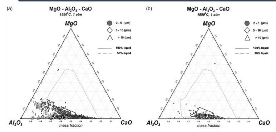
Elemental chemical composition of inclusions detected by SEM-EDS plotted in ternary diagrams for the MgO–Al<sub>2</sub>O<sub>3</sub>–CaO system. a) Before the industrial process changes (2800 inclusions). b) After the industrial process changes (1470 inclusions).
