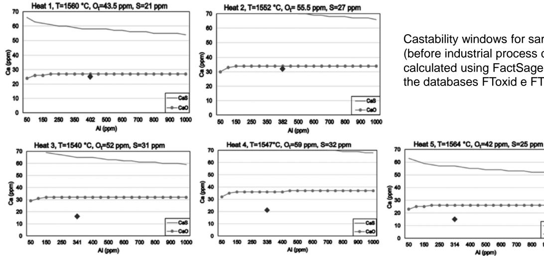
Castability windows for samples 1–5 (before industrial process change) calculated using FactSage 7.1 with the databases FToxid e FTmisc.
