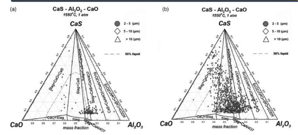
Elemental chemical composition of inclusions detected by SEM-EDS plotted in ternary diagrams for the CaS–Al<sub>2</sub>O<sub>3</sub>–CaO system. The number of CaS-bearing inclusions dramatically increased.
