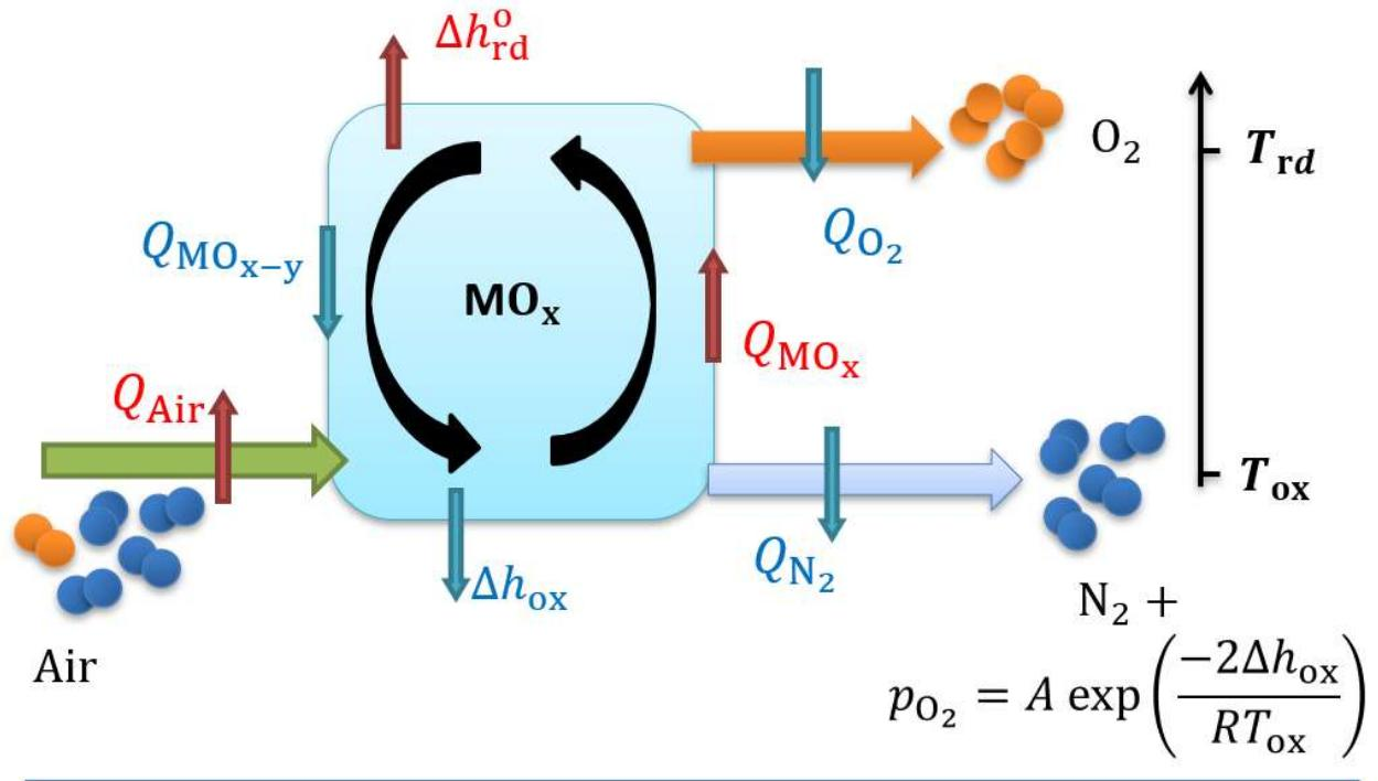
$$Q_{\text{in}} = 2\Delta h_{\text{rd}}^{\circ} + Q_{\text{Air}} + Q_{\text{MO}_x} = Q_{\text{out}} = 2\Delta h_{\text{ox}} + Q_{\text{O}_2} + Q_{\text{N}_2} + Q_{\text{MO}_{x-y}}$$
