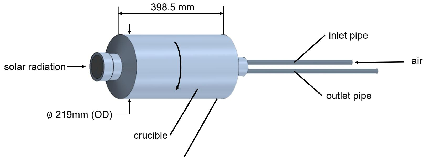
thermal insulation is considered as adiabatic wall (adiabatic wall does not allow the transfer of heat)
