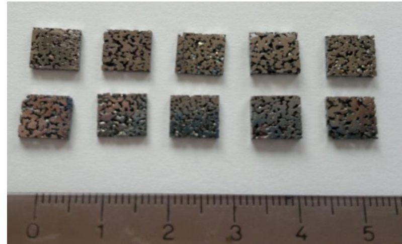
Representative porous SHS NiTi sample for biological tests
