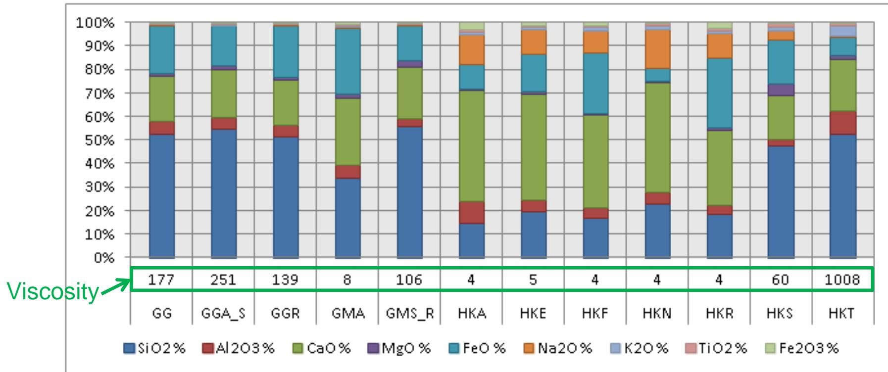
Composition of the slag at the temperature where 40% of liquid phase are reached
