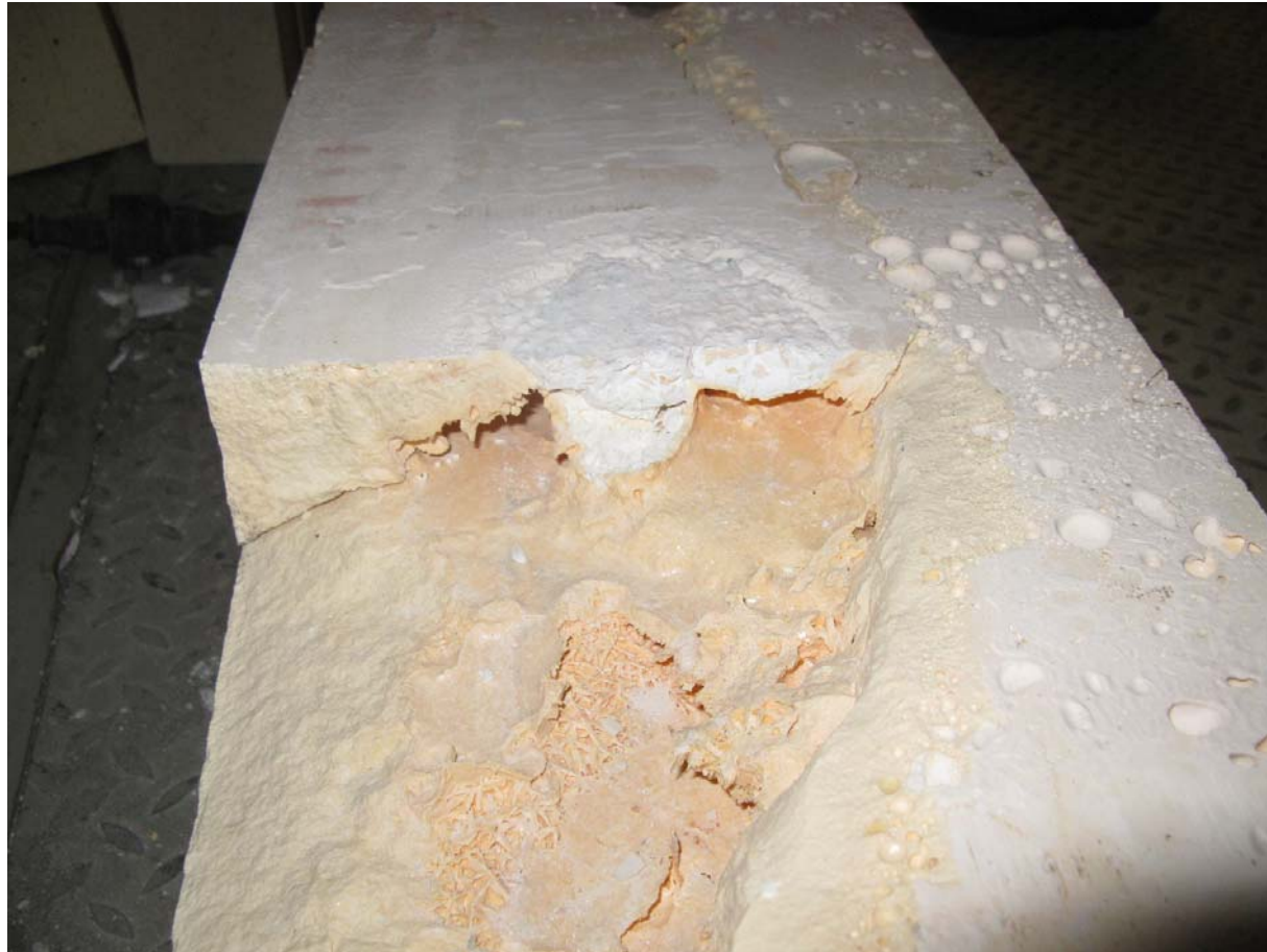
Damage of a Brick by steam explosion / pers. memo. D. Lenzner (2012)
