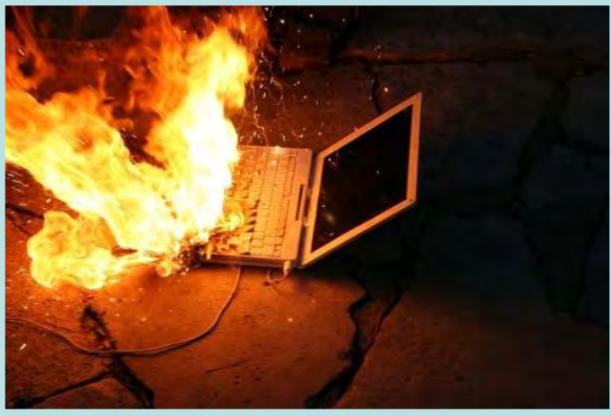
Rechargeable battery of a laptop – overheating or internal short circuit
