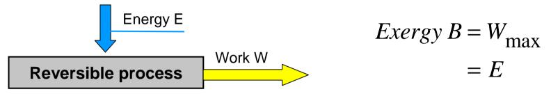
• Thermal energy can only partially transformed into work (Carnot-law)
