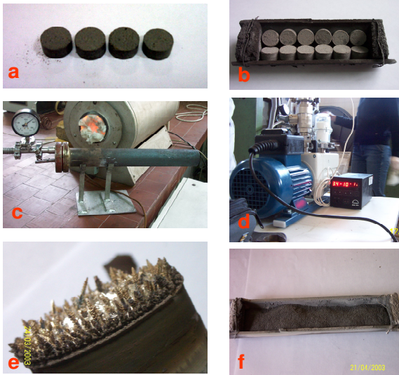
Fig. 6 a) Briquetted Charges b) Boat with Briquettes c) Reduction Retort and Furnace d) Vacuum Pump e) Collected Magnesium f) Residue after an experiment
