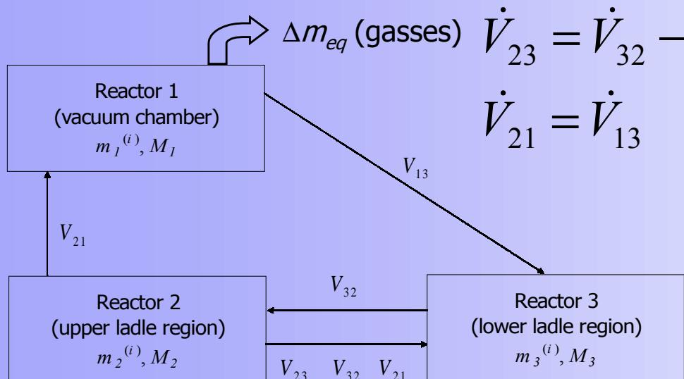
$m_i$  – mass of reactant in  $i^{\text{th}}$  reactor, [Mg],
